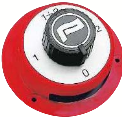
Battery master switch 17540 Suitable for one or two battery installations : to isolate or cluster the lighting and engine start circuits. Capacity 150 A/12 V. Polycarbonate case, footprint Ø 134 mm, height 65.7 mm. Easy surface mounting, supplied with instructions. Knob Ø : 52 mm.
