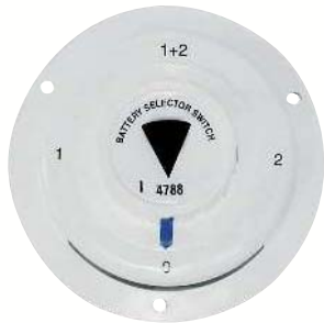
Battery coupler 417678 Rated 250 A continuous, 300 A-12 V intermittent. Allows changing batteries without switching off the engine. Dimensions : Ø 145 x 67 mm. Knob Ø : 57 mm.
