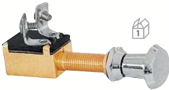
Pull switch 402754 2-position chromed switch - 3 contact plates Ø 9 mm, overall length 95 mm. 12 V - 15 A.
